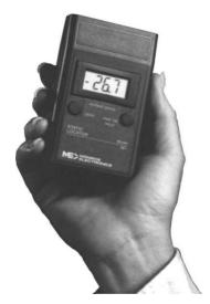
**NOTE** — If, as you approach the target, the indicated field strength begins to exceed 20kV at a distance greater than 1", **STOP!** This implies that the target voltage may be high enough to create an arc. Proceed with caution.
